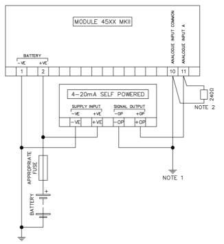
NOTE 1. THESE GROUND CONNECTIONS MUST BE ON THE ENGINE BLOCK, AND MUST BE TO THE SENSOR BODIES.
