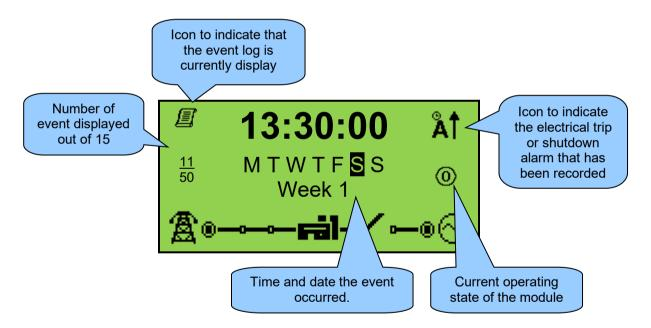
The events shown in the below table are recorded into the module's event log in addition to all electrical trip and shutdown alarms.
