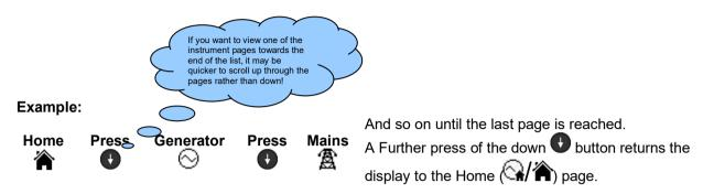
Once selected, the page will remain on the LCD display until the user selects a different page or, after an extended period of inactivity (*Page Delay Timer*), the module reverts to the Home (A) page.
